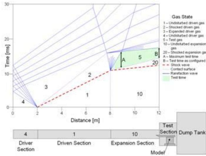
Figure 1: Distance versus time (x-t) diagram showing the configuration of a generic expansion tube and the processes that occur during a test
