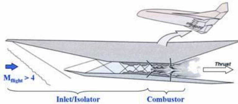
Figure 6: Generic scramjet showing the complex inlet shock system
