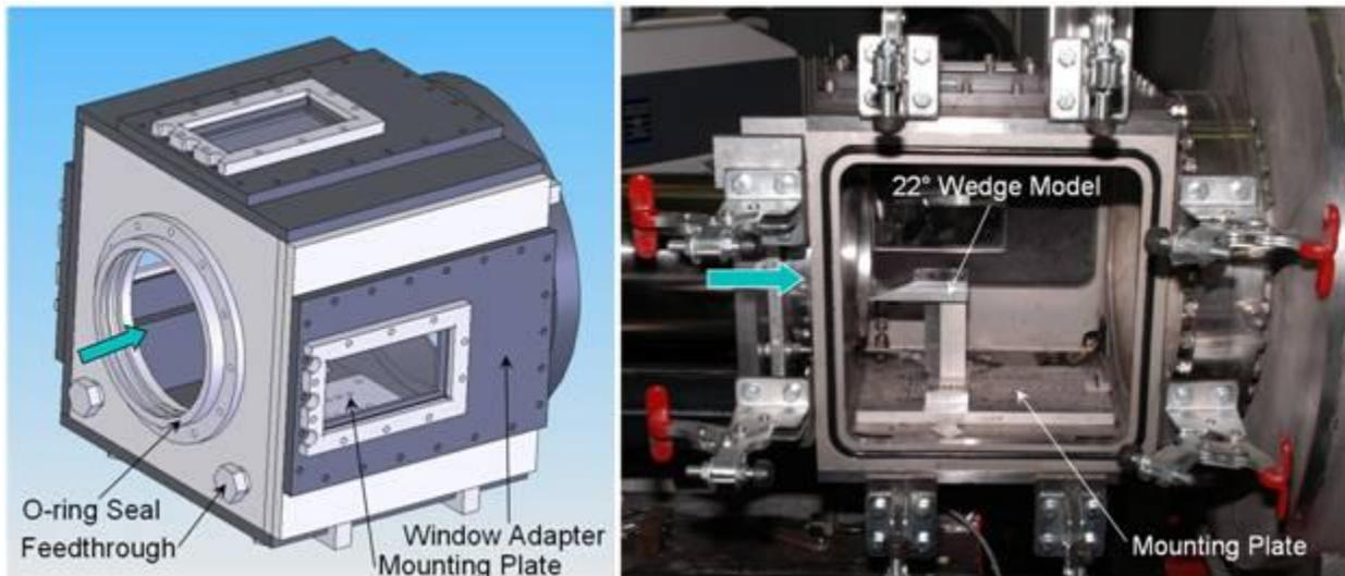
Figure 4: Test section. Solid model (a) and photograph (b) with the access cover removed and a 22° wedge model installed for Schlieren imaging.
