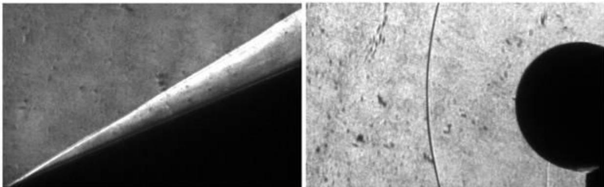
Figure 5: Example Schlieren images as used for facility characterization with (a) a 22° wedge indicating flow at Mach 6.3 and (b) a circular cylinder indicating flow at Mach 1.85.
