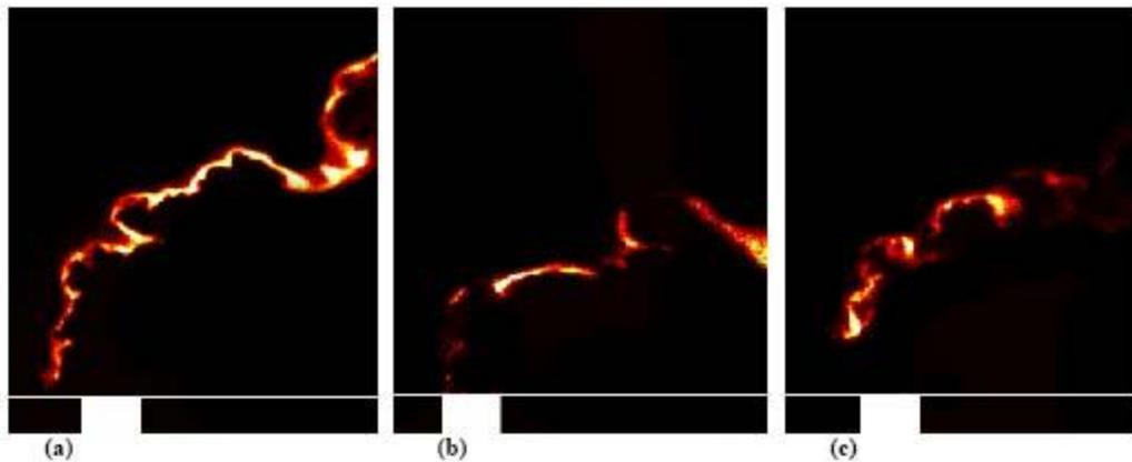
Figure 8: OH PLIF images of various regimes of burning: (a) strong combustion at  $T_0 = 3100$  K,  $T = 1375$  K,  $P = 25$  kPa and  $J = 4$  (b) patchy combustion at  $T_0 = 2500$  K,  $T = 1375$  K,  $P = 25$  kPa and  $J = 2$ , and (c) combustion with extinction at  $T_0 = 2500$  K,  $T = 1375$  K,  $P = 25$  kPa and  $J = 4$ . The jet diameter and plate surface in each image are as marked, and all images are corrected for incident laser sheet intensity.
