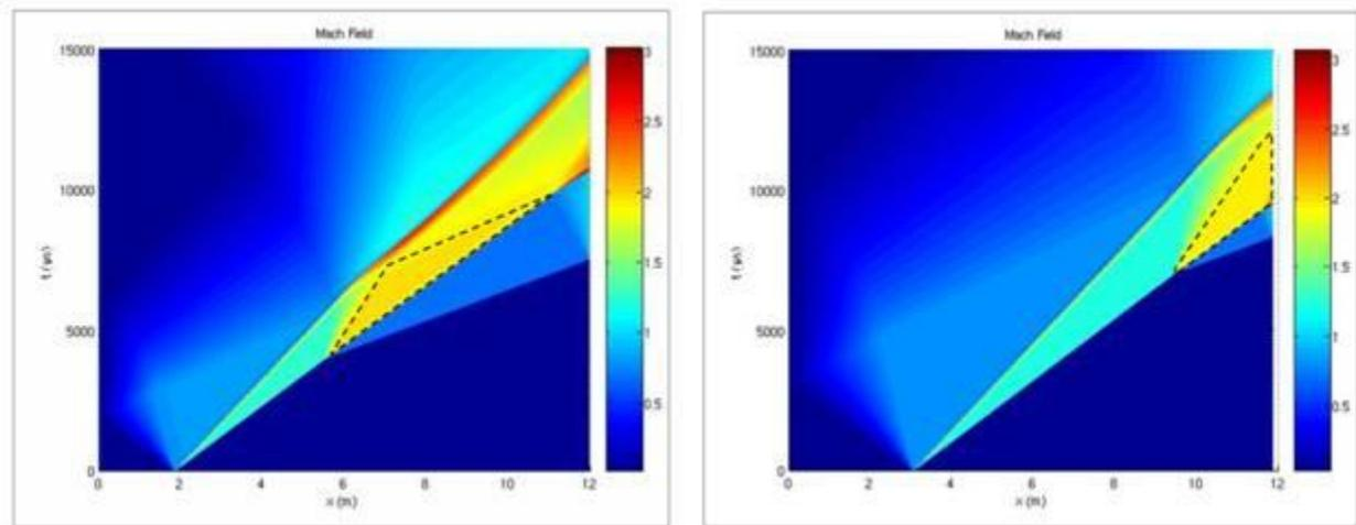
Figure 2: 1-D inviscid model of an expansion tube with varying tube layout. With the primary diaphragm located 2 meters from the endwall and (a) the secondary diaphragm located 5.7 meters from the endwall, the test gas, shown as a black triangle, does not reach the tube exit. However, (b) by moving the secondary diaphragm to 9.7 meters, the test gas reaches the tube end and useful test time is obtained.
