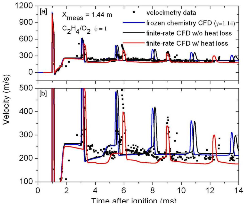
Figure 3: Velocimetry data for converging-diverging nozzle configured PDE plotted against model data. Window [b] shows a region of window [a] with the vertical axis rescaled
