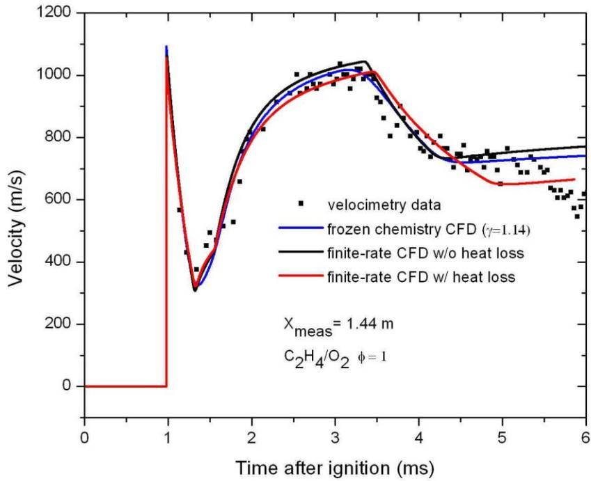
Figure 2: Velocimetry data for straight-tube PDE plotted against model data
