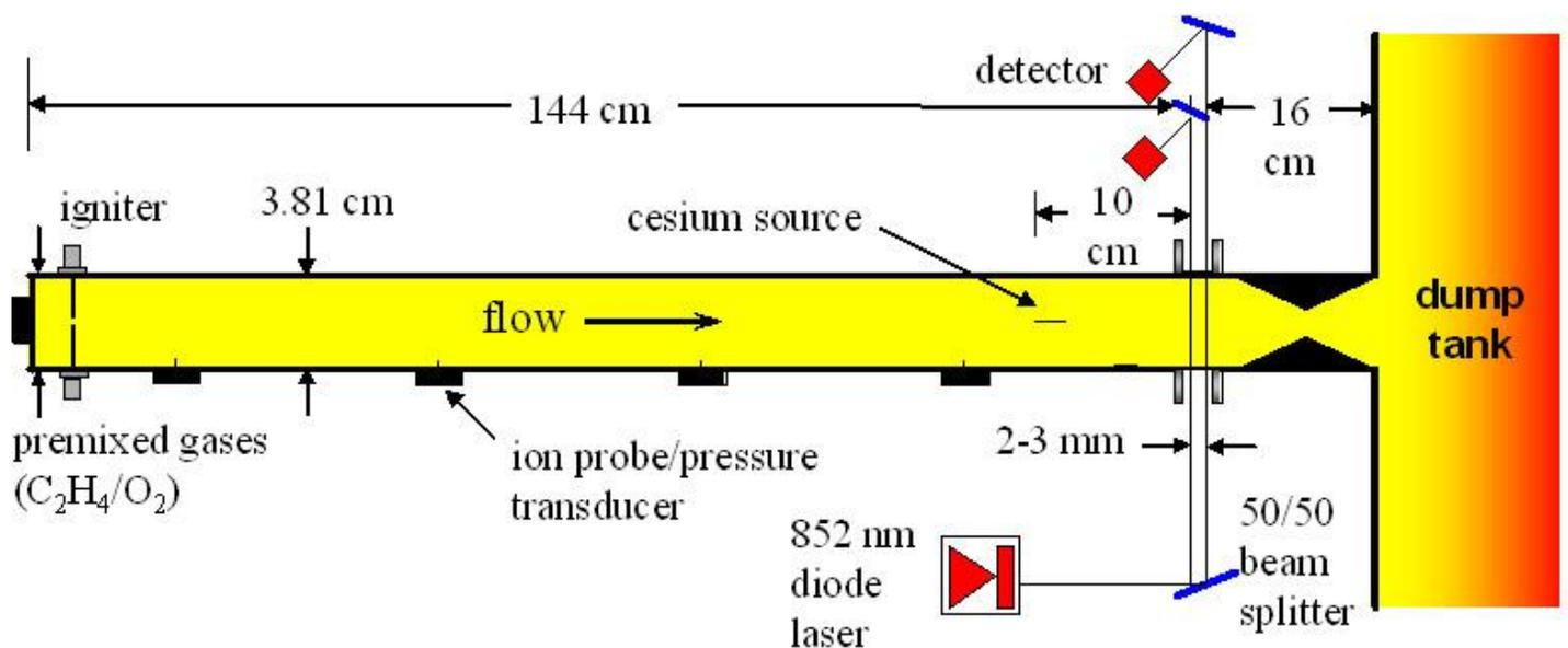
Figure 1: Schematic of Stanford PDE facility with cesium-based velocimetry diagnostic
