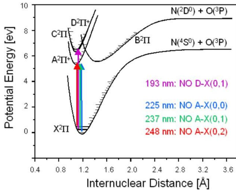
Figure 2: NO potential diagram for excitation scheme
