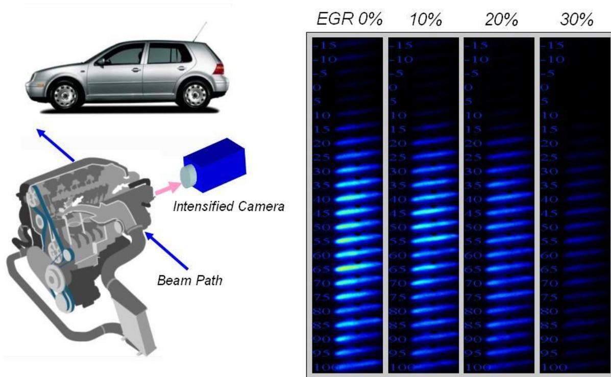
**Figure 6: Quantitative NO-LIF imaging in internal combustion engine**
