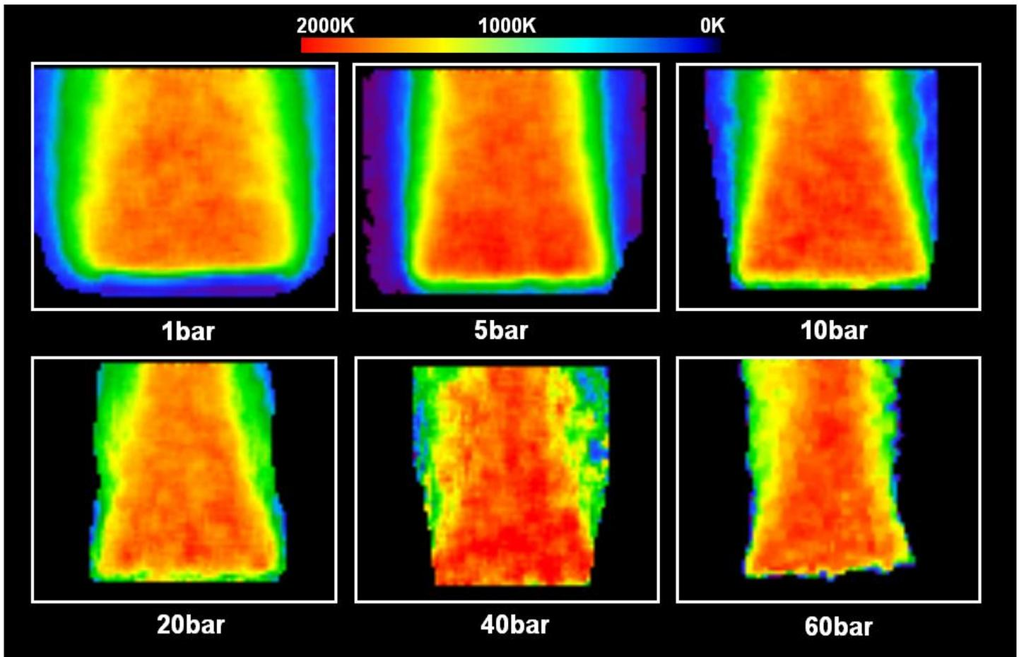
Figure 4: Temperature field Imaging using A-X(0,0) NO PLIF
