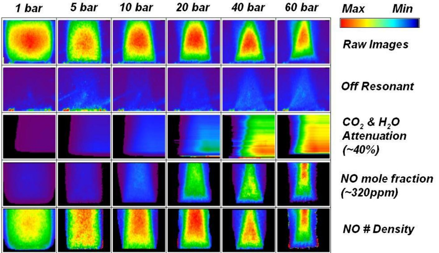
Imaging Results from A-X(0,0) transition at 225nm
