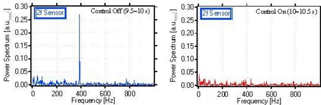
**Figure 2: FFT power spectra with and without control.**
