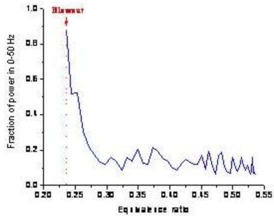
Figure 3: Fraction of FFT power in 0-50 Hz of the T-sensor output signal as a function of equivalence ratio.
