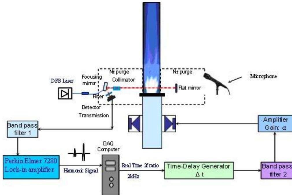
**Figure 1: Experiment setup for suppressing thermoacoustic instability using real-time T-sensor.**
