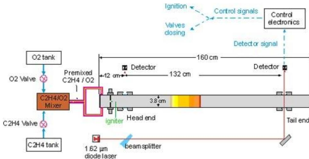
Figure 3: Schematic of C2H4 sensor applied to Stanford PDE for monitoring and control.
