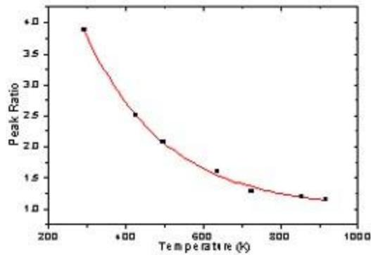
Figure 2: Ratio of the two peaks indicated in Figure 1 showing sensitivity of temperature sensor.
