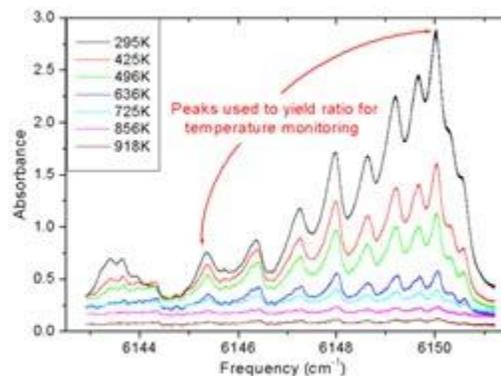
**Figure 1: Q-branch of  $C_2H_4$  near 1.62 mm at different temperatures.**
