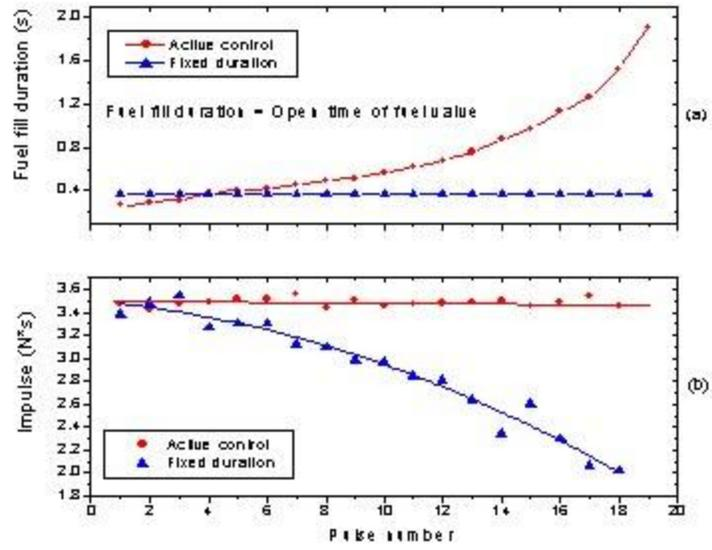
Figure 4: Demonstration of active control using a diode laser sensor to optimize fuel consumption and achieve uniform impulse per PDE cycle. (a) comparison of fuel fill duration, and (b) comparison of impulse per cycle between fixed duration case and active control case
