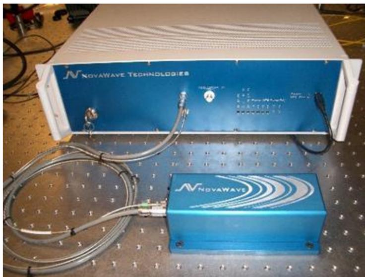
**Figure 1: Tunable mid-IR laser used for sensitive hydrocarbon detection.**
