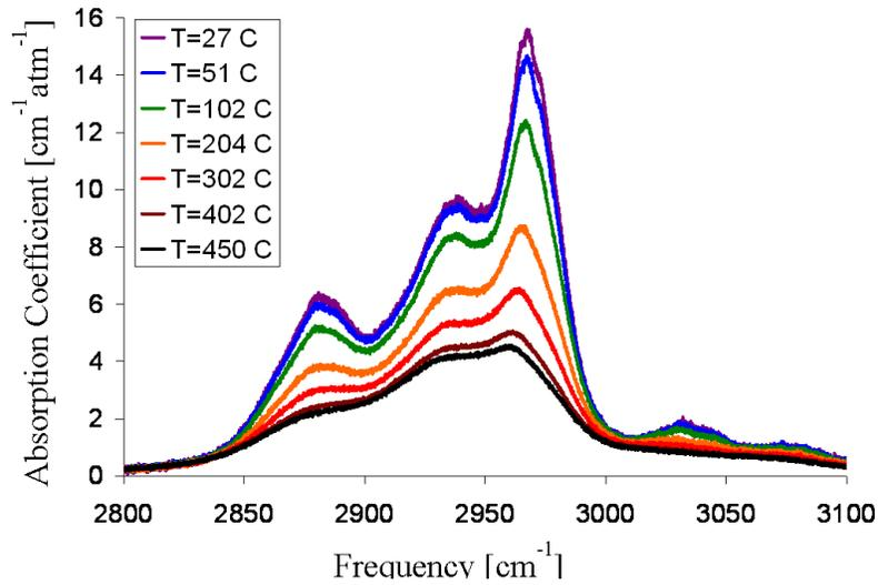
**Figure 2: Temperature-dependent absorption cross section of regular grade gasoline measured by FTIR.**
