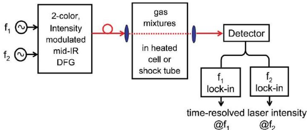
Figure 4: Experimental setup for absorption measurements of hydrocarbon fuel with two-color, intensity-modulated sensor
