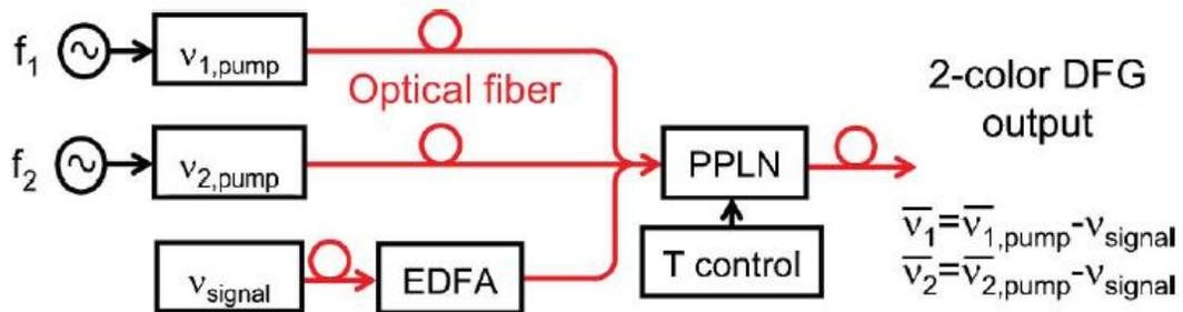
**Figure 3: DFG scheme for simultaneous production of two mid-IR laser frequencies at  $\nu_1$  and  $\nu_2$  with intensity modulation at  $f_1$  and  $f_2$**
