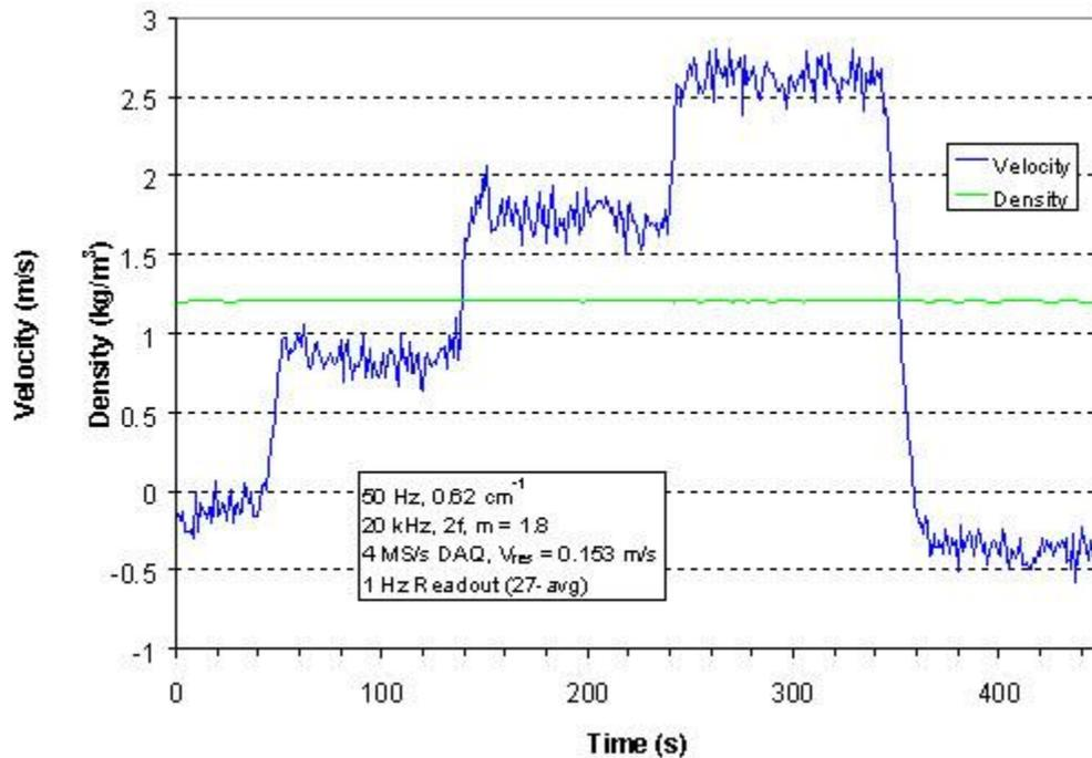
Figure 5: Timeline of velocity in a low speed wind tunnel, with real-time readout rate of 1 Hz.
