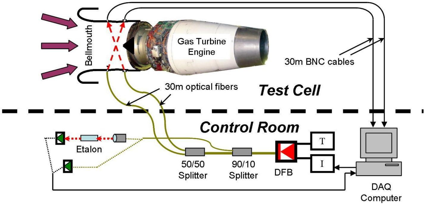
Figure 6: Schematic of an air mass flux sensor installed on the inlet of a commercial jet engine, (Airbus 318).
