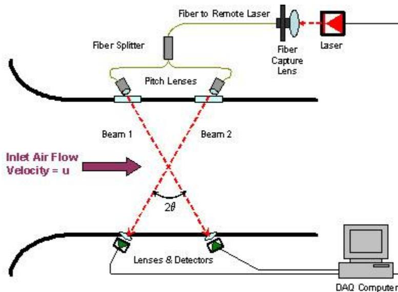
Figure 3: Schematic of mass flux sensor using split paths to measure Doppler shift for velocity measurement.
