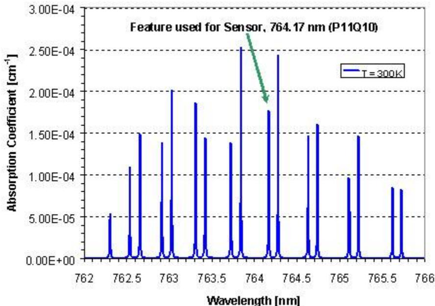
**Figure 1: Spectral absorption coefficient vs. wavelength for P-branch of O2 A-band, T = 300K.**
