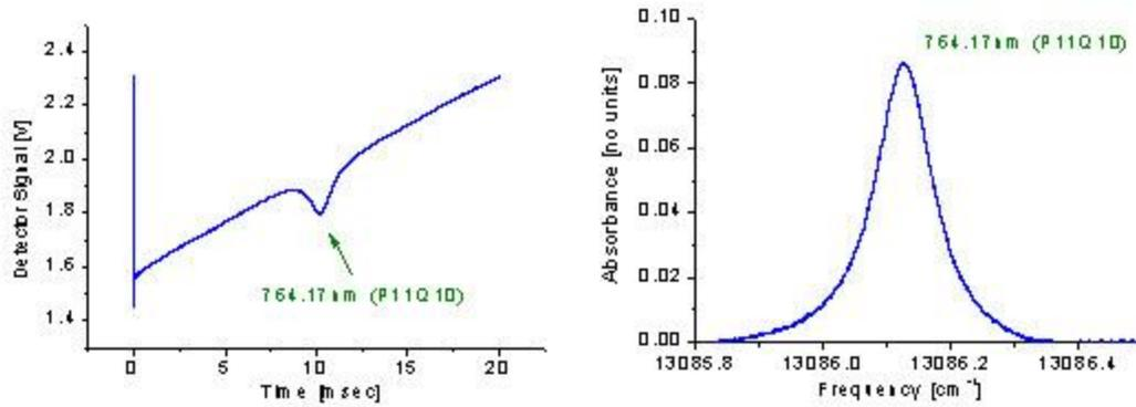
Figure 2: Linear diode laser scan across O2 absorption feature (left). Absorbance of same scan using absorbance =  $-\ln(I/I_0)$  (right).
