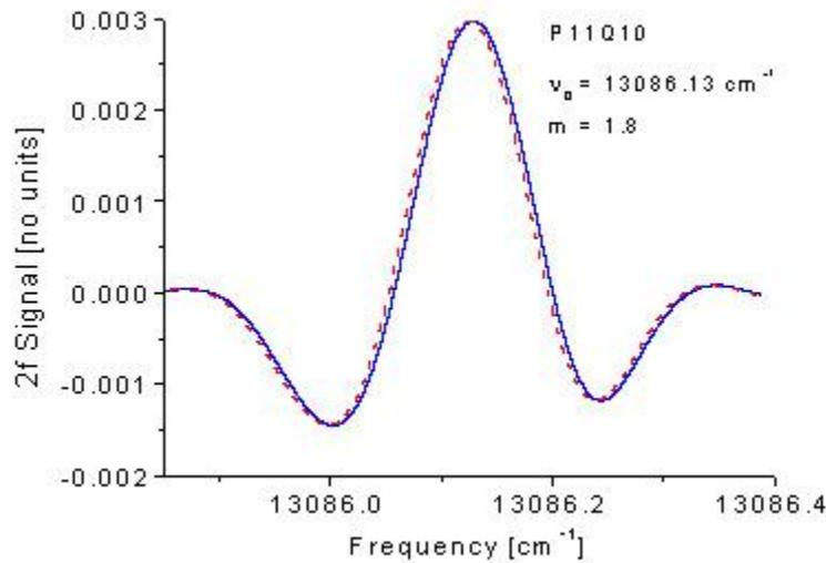
Figure 4: Two 2f lineshapes Doppler shifted by a velocity of 100 m/s (theta = 30°).
