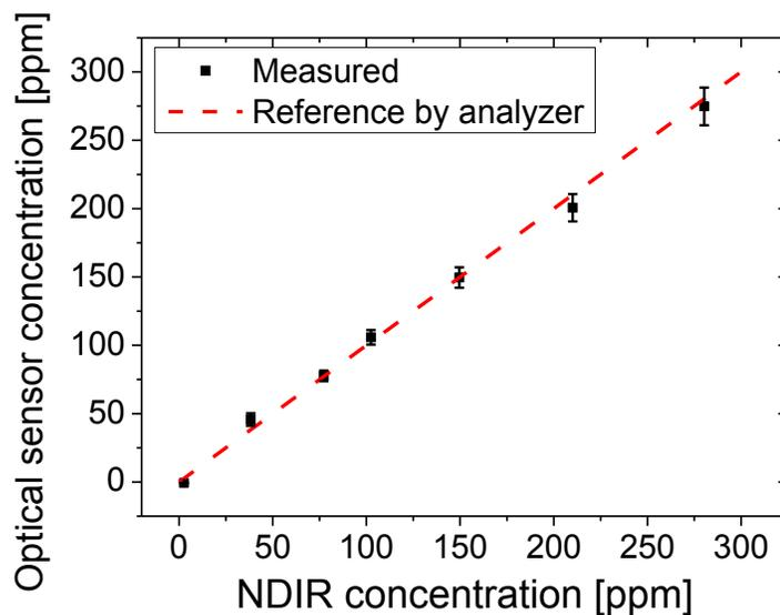
**Figure 3: Concentrations measured by 2f/1f optical sensor versus NDIR measurement in sampled combustion gas with pathlength L=1.79m.**
