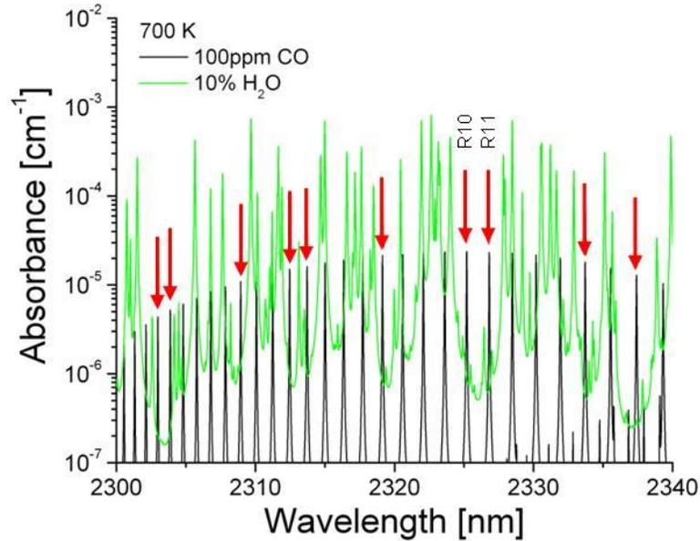
**Figure 2: Absorbance per cm of pathlength for 100ppm CO and 10% H<sub>2</sub>O at 800 F (700 K) in atmospheric pressure gas simulated from HITRAN. Transitions for CO sensing with the potential to avoid H<sub>2</sub>O interference are marked with red arrows; transitions R(10) and R(11) are especially promising. (Simulation calculation from HITRAN)**
