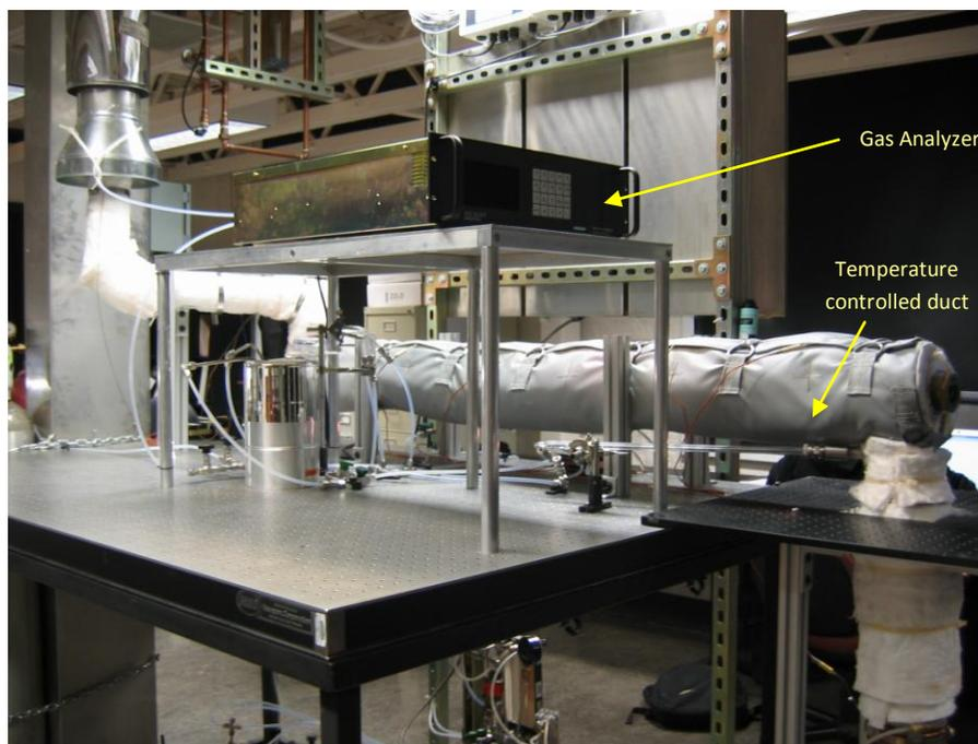
**Figure 1: Stanford's constant temperature combustion exhaust duct facility**
