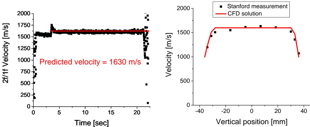
**Figure 4: Measurements of velocity in the DCSCF during a measurement campaign at NASA Langley in September 2009. Left panel: velocity versus time is quite stable after initial transient; Right panel: velocity versus vertical position in good agreement with CFD prediction with potentially a slightly thicker boundary layer.**
