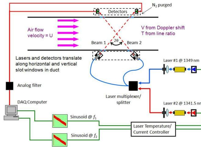
**Figure 2:** Two-laser frequency-multiplexed WMS sensor for mass flux at  $\text{H}_2\text{O}$  wavelengths  $\lambda_1$  and  $\lambda_2$  ( $\sim 1349$  and  $1341.5$  nm). The two lasers are combined on a single fiber and then split to be directed upstream and downstream in the supersonic flow with a crossing angle  $2\theta$ . Velocity is determined from Doppler shifts of the absorption lineshape and gas temperature by the ratio of the two absorption signals.
