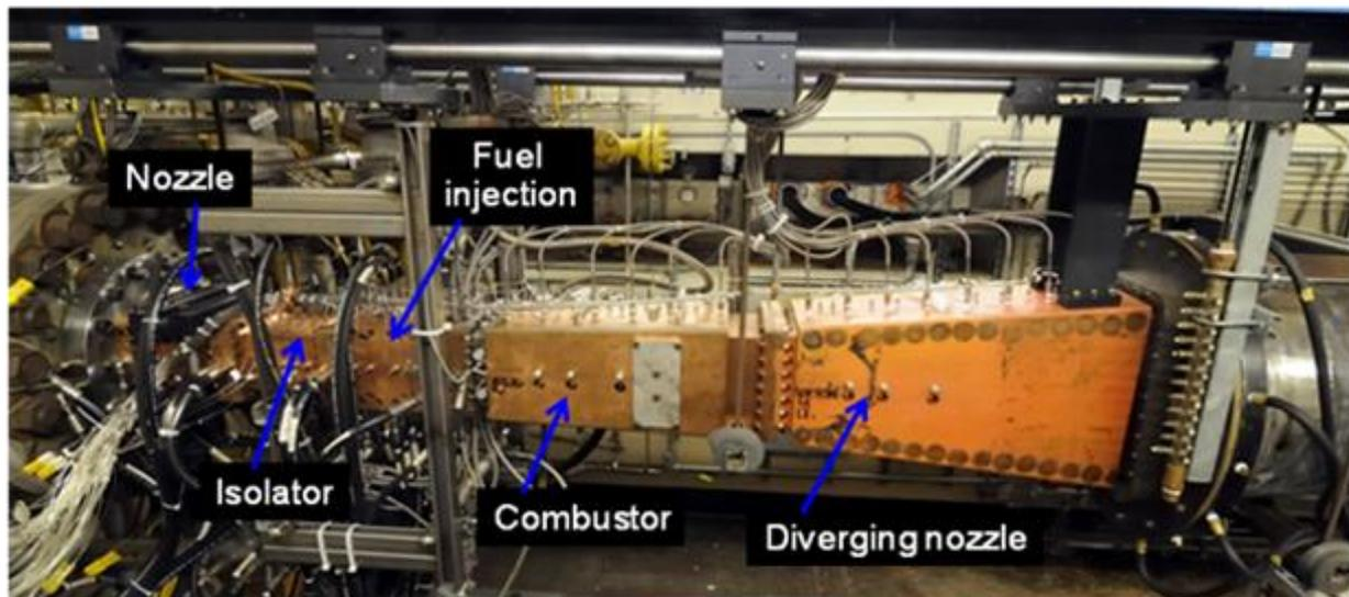
Figure 1: NASA Langley Direct Connect Supersonic Combustion Test Facility (DCSCTF).
