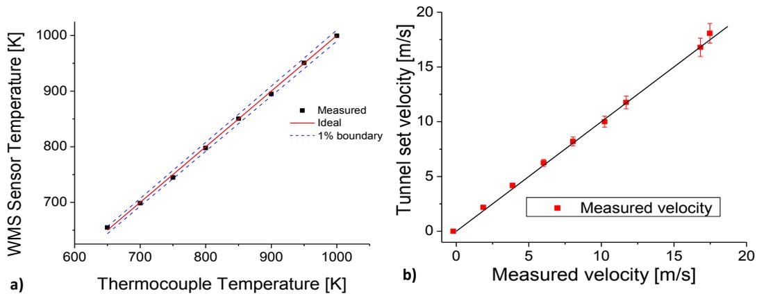
**Figure 3:** a) Sensor temperature measurement in Stanford high-uniformity furnace. b) Sensor velocity measurement in Stanford low speed wind tunnel.
