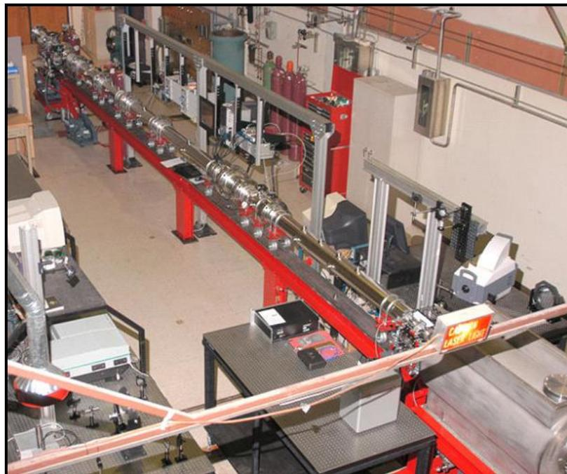
**Figure 1: Stanford Expansion Tube Flow Facility capable of reproducing the thermodynamic and aerodynamic conditions of a scramjet combustor flow.**
