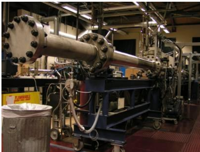
Figure 1: Aerosol shock tube
