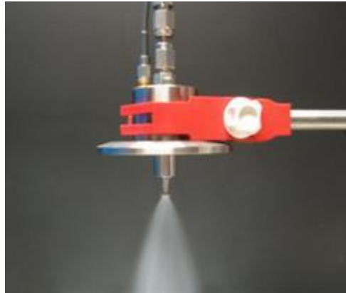
Figure 2: Sonotek ultrasonic spray nozzle in operation in our laboratory
