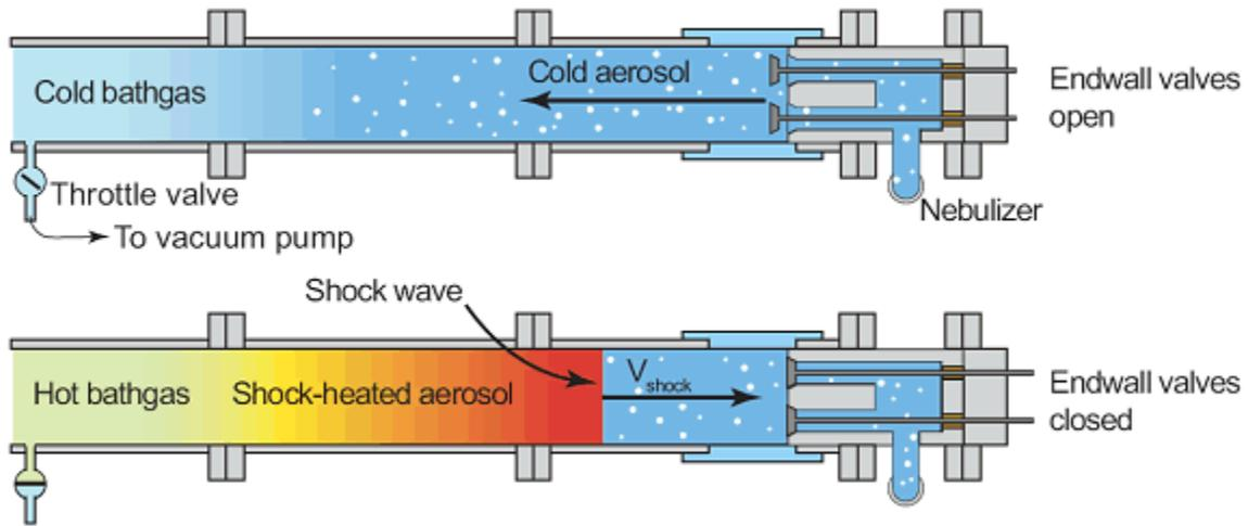
Figure 4: Aerosol shock tube filling and shocking
