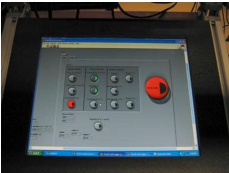
**Figure 11: Touch-screen control panel**
