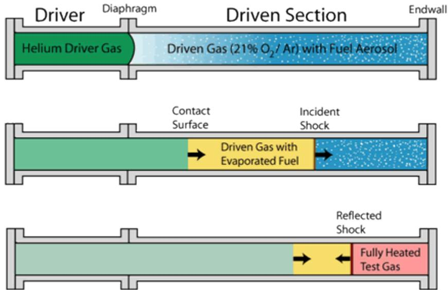
**Figure 2: Aerosol shock tube operation**
