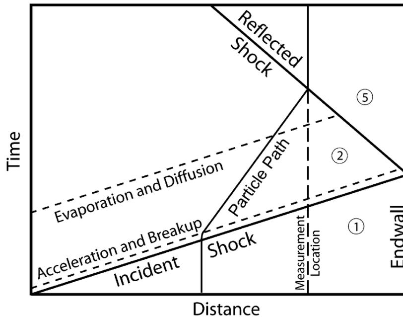
Figure 5: Aerosol shock tube x-t diagram [ref 1]
