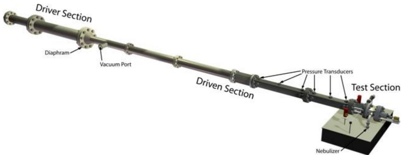
**Figure 1: CAD drawing of aerosol shock tube**
