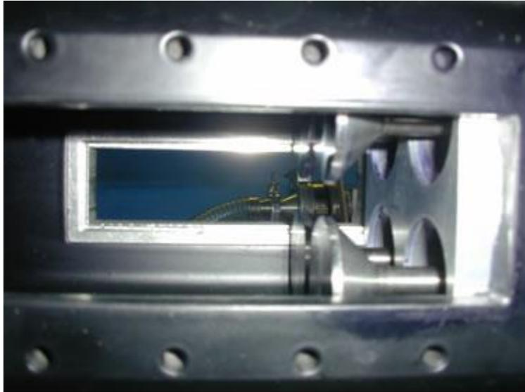
**Figure 8: View of open poppet valves within shock tube**
