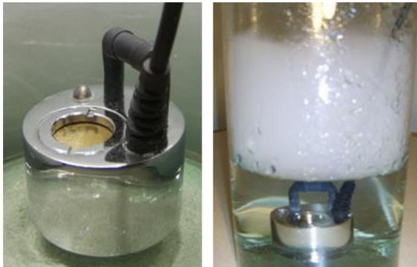
**Figure 3: Ultrasonic nebulizer, made by Ocean Mist**
